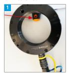
c. Pump oil into the hydraulic nut until oil emerges without air bubbles at the ball pressure plug
